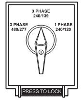
Figure 16. Voltage Selector Switch
